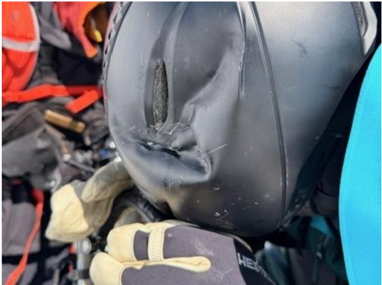
The helmet of the injured party showed significant damage from the falling object (rock or ice).
